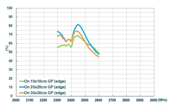
Figure 7. Efficiency of WCM.01 on edge of different ground plane sizes
