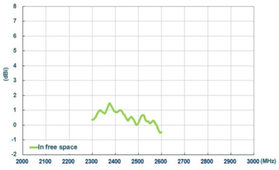
Figure 8. Peak gain of WCM.01 antenna in free space
