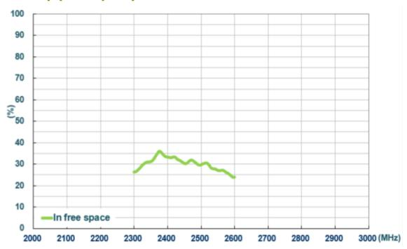
Figure 5. Efficiency of WCM.01 antenna in free space
