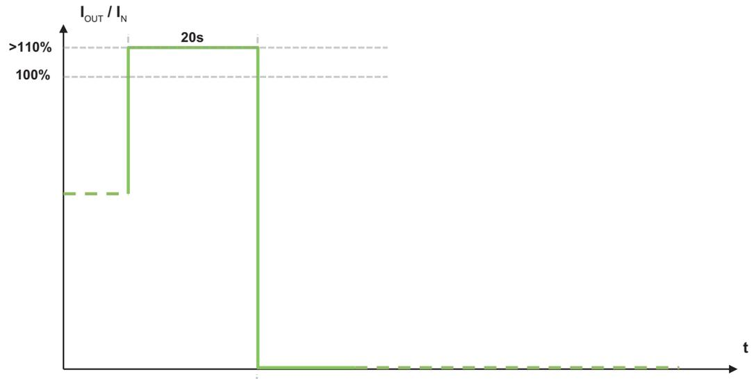
Figure 40: "Constant Current with Latching Shutdown" Mode
