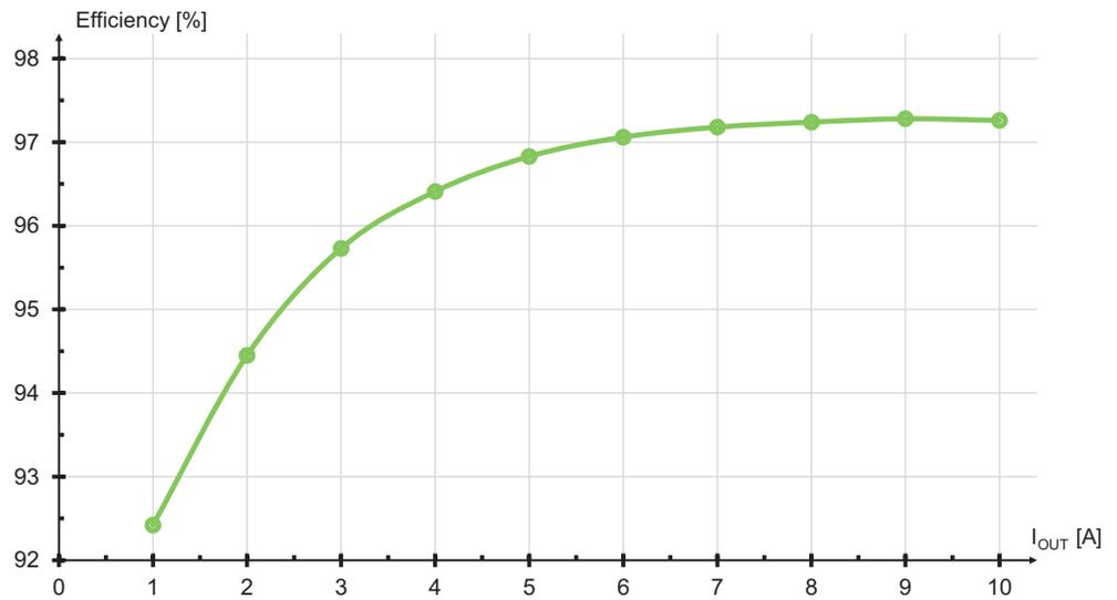
Figure 11: Efficiency (typ.) at 400 VAC
