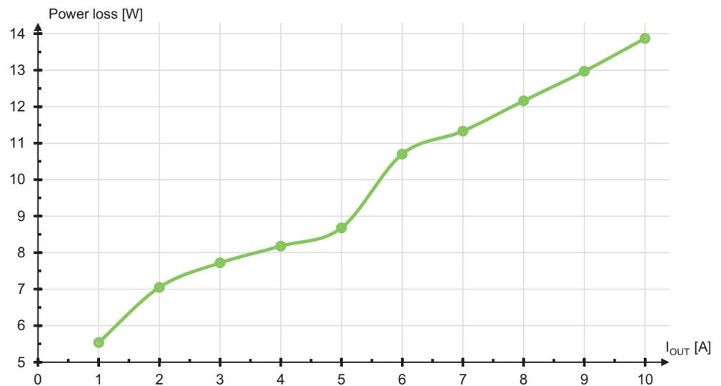
Figure 12: Power loss (typ.) at 400 VAC
