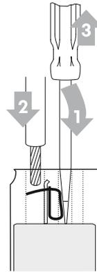
Figure 17: Connect Conductor to CAGE CLAMP®
