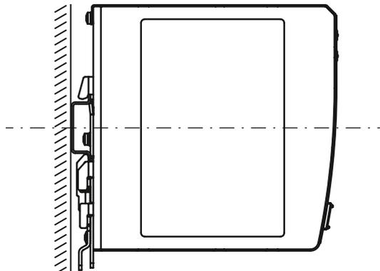
Figure 14: Position of the DIN-35 rail
