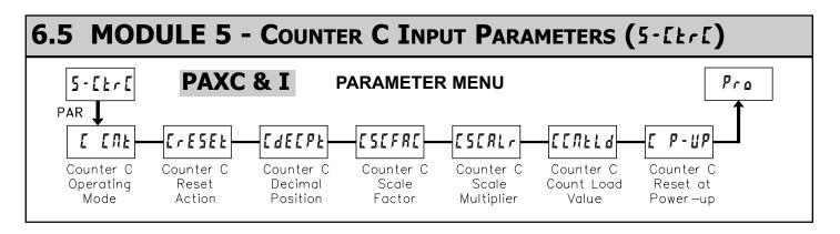
Module 5 is the programming for Counter C. For maximum input frequency, the counter operating mode should be set to **Pape** when not in use. When set to **Pape** the remaining related parameters are not accessible. The C annunciator indicates that Counter C is being shown in the Display Mode. An Exchange Parameter List feature for scale factor and count load values is explained in Module 2.
