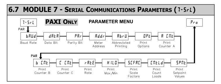
Module 7 is the programming module for the Serial Communications Parameters. These parameters are used to match the serial settings of the PAXI with those of the host computer or other serial device, such as a terminal or printer. This programming module can only be accessed if an RS232 or RS485 Serial Communications card is installed.
