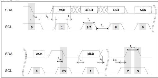
$<sup>^{\</sup>star\star}$ ) For I<sup>2</sup>C bus capacitance load >100pF maximum possible clock frequency is 100kHz
