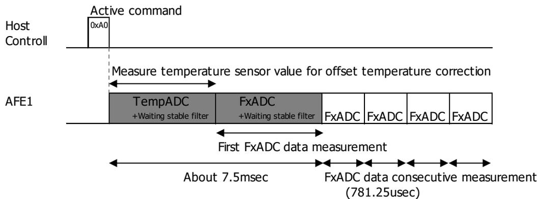
Fig. 10 Schematic of AD conversion start instruction
