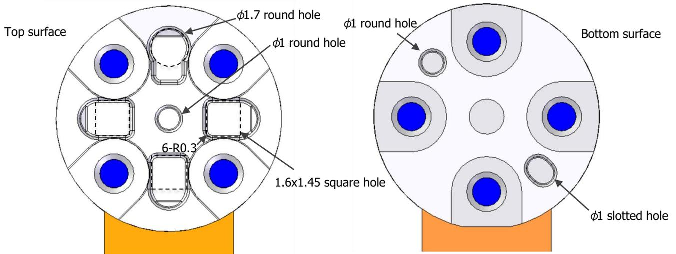
Fig. 30 Positioning holes
