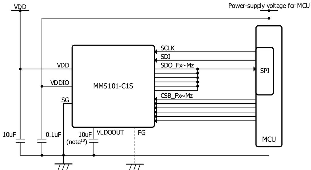
Fig. 23 Integrated SDO pin – Example application circuit
