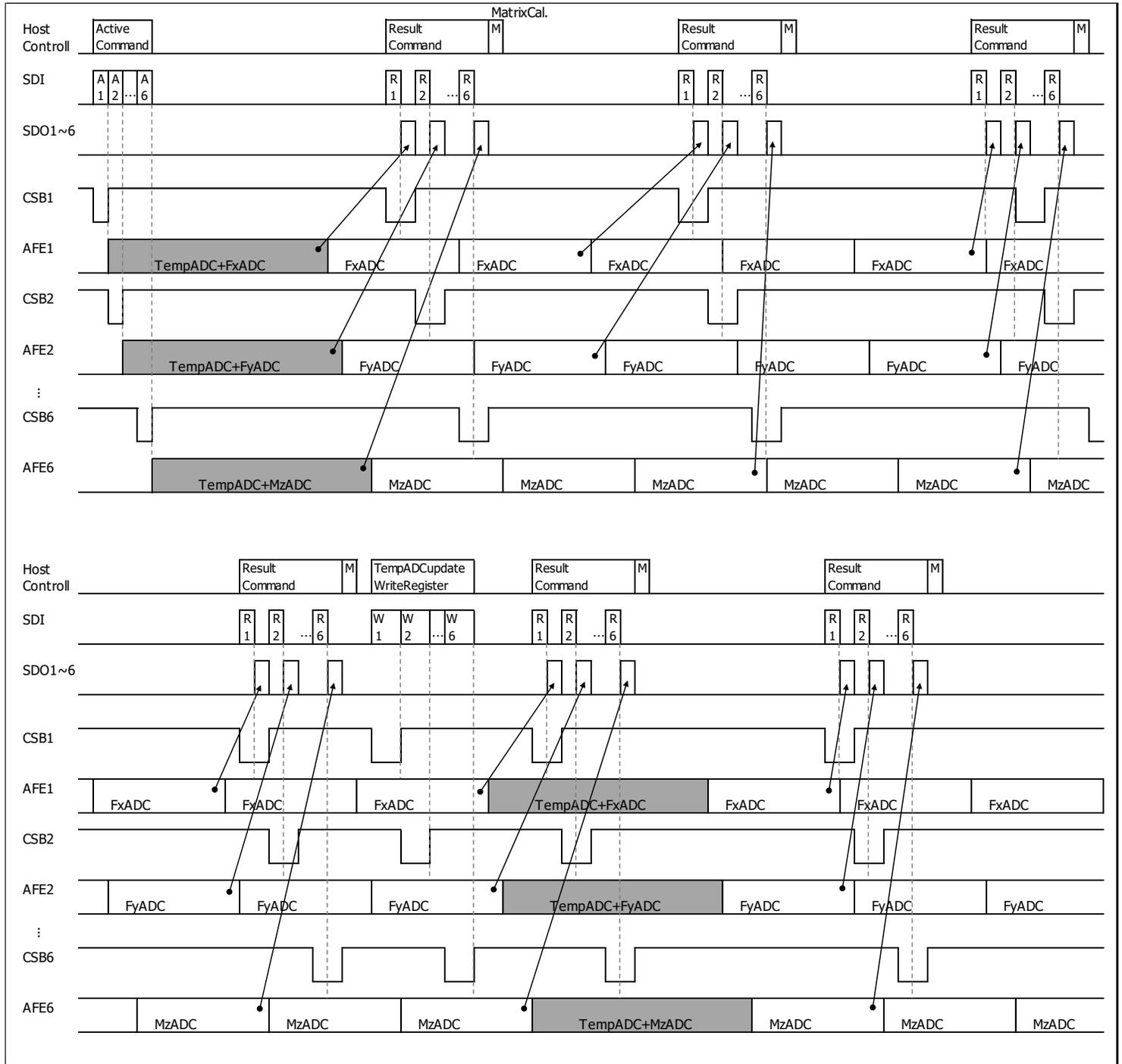
\*AD conversion cycle depends on AFE because internal clock is different from each AFE.
