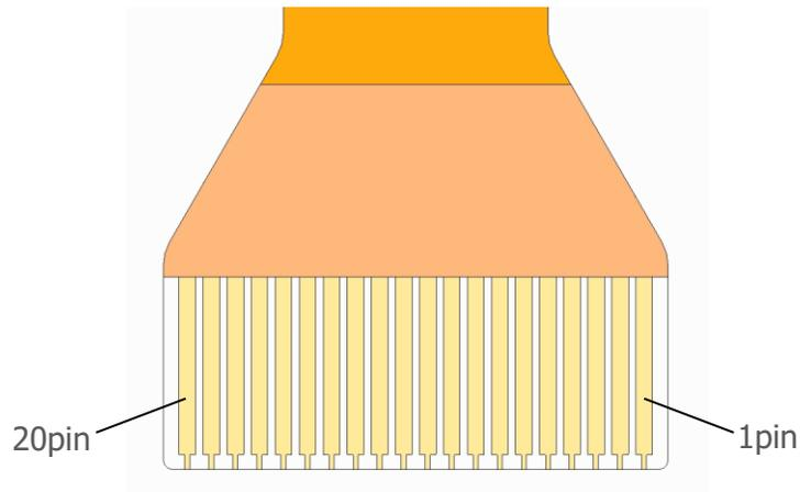
Fig. 3 Pin configuration
