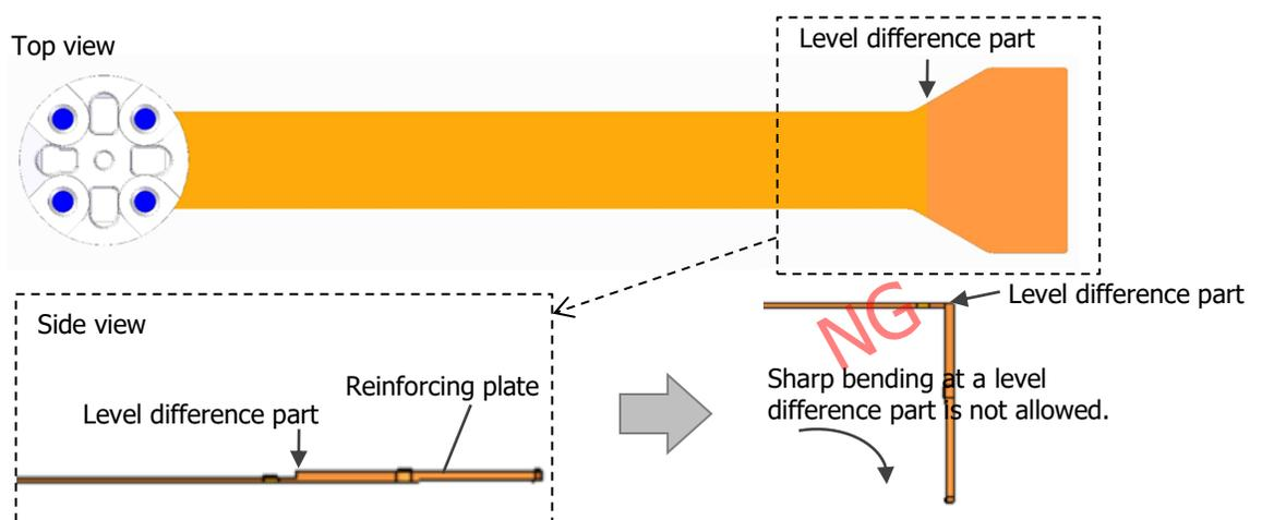
Fig. 34 Precaution for handling of sensor FPC - 2
