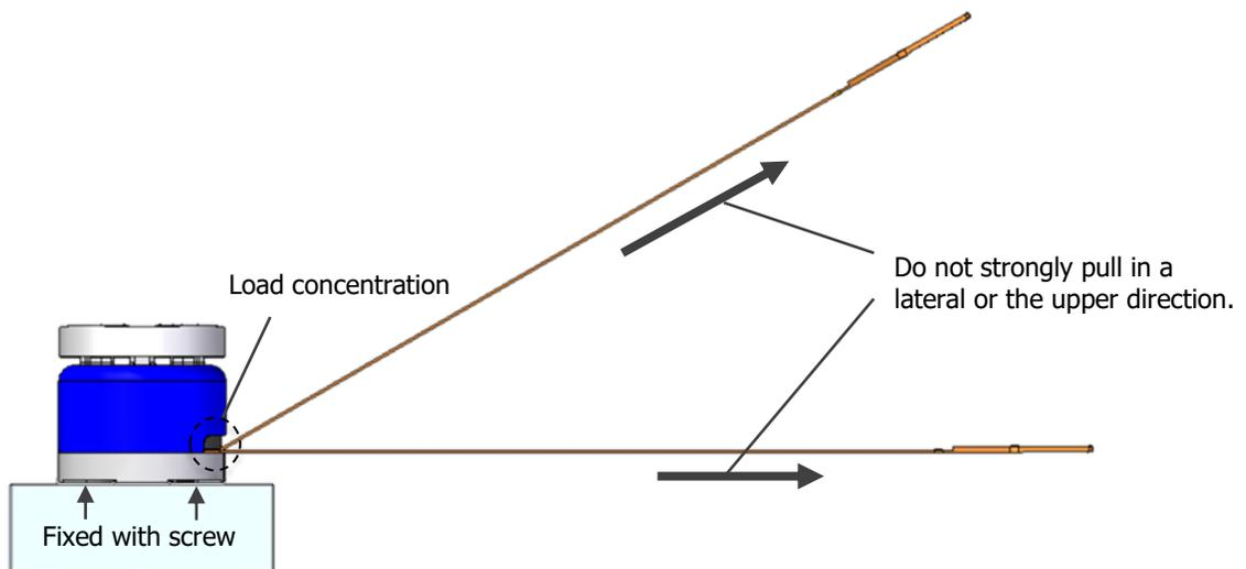
Fig. 33 Precaution for handling of sensor FPC - 1
