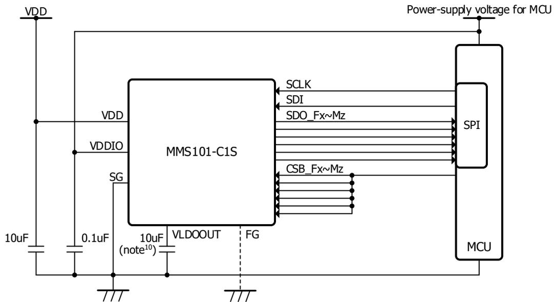
Fig. 22 Integrated CSB pin – Example application circuit
