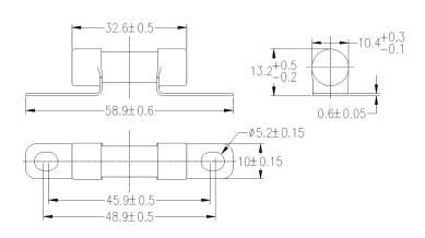
Note: recommend tightening torque is 3.5-4 Nm for M5 screw
