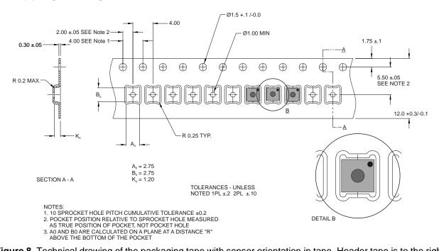
**Figure 8.** Technical drawing of the packaging tape with sensor orientation in tape. Header tape is to the right and trailer tape to the left on this drawing. Dimensions are given in millimeters.
