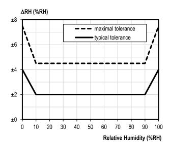
Figure 1. Maximal and typical tolerance of RH at 25°C
