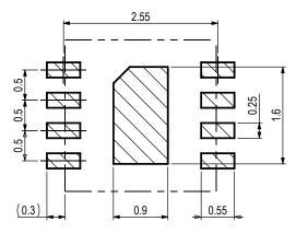
**Figure 7.** Recommended metal land pattern (left) and stencil apertures (right) for SHT33-DIS. The dashed lines represent the outer dimension of the DFN package. The PCB pads (left) and stencil apertures (right) are indicated through the shaded areas.
