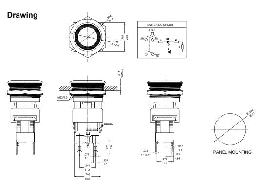
Note: Tolerances Unless Otherwise Specified:± .012/0.3 (in/mm)
