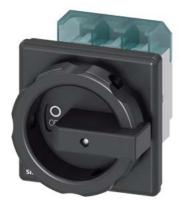
SENTRON, Switch disconnector 3LD, main switch, 3-pole, lu: 63 A, Operating power / at AC-23 A at 400 V: 22 kW, front-mounted, rotary operating mechanism, black, 4-hole mounting of the handle
