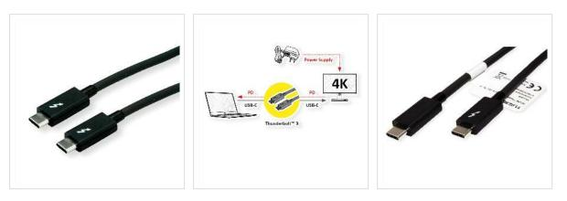
Thunderbolt 3 cables with the USB Type C connector offer you the currently highest possible data transfer rate of up to 40GBit/s (20GBit/s for 1m and 2m) and full Power Delivery support (PD up to 20V 5A / 100W)! The cables also feature DP mode for particularly high-resolution image and sound transmission of up to 5120x2880 @60Hz (5K).
