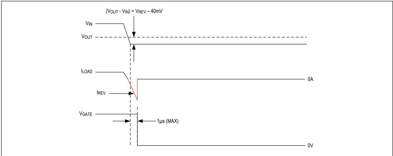
Figure 3. Reverse-Voltage Fault
