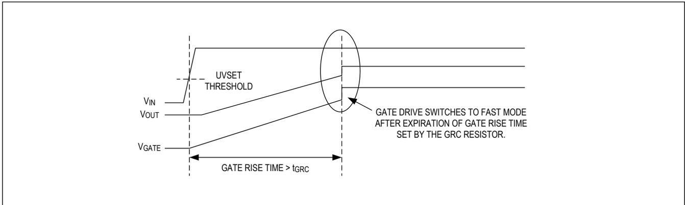
Figure 6. Gate Voltage Slow to Fast-Mode Transition
