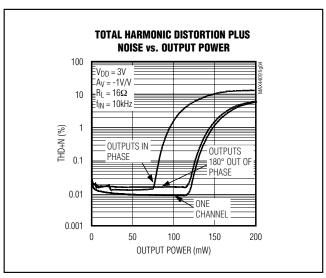
Figure 4. Output Power vs. THD+N with Inputs In/Out of Phase
