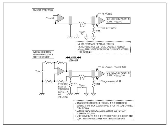
Figure 6. Common-Mode Noise Rejection
