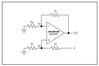
Figure 5. Common-Mode Sense Equivalent Circuit
