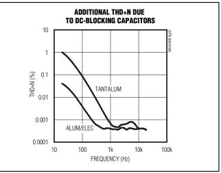
Figure 3. Distortion Contributed by DC-Blocking Capacitors
