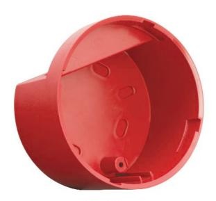
The bayonet base has been designed to allow a common mounting for most of Fulleon's conventional alarm products. The Shallow Base is suited to concealed wiring allowing installation with minimum visual impact. The deep and "U" bases cater for surface wiring of all types and provides ingress protection up to IP65. Combinations of two or more Deep bases form the basis of the AV Unit allowing for many permutations of audible and visual warning units.
