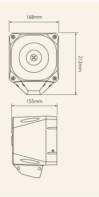
The Asserta Industrial warning sounder / beacon is designed to cope with harsh environments requiring protection to IP66. Design features are incorporated to ensure safer and easier installation, while providing flexibility with fewer product variants.
