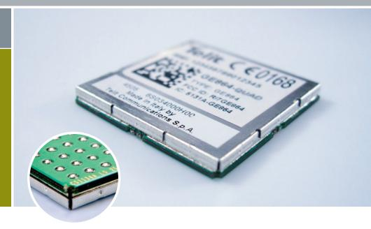
The new GE864 product family introduces the smallest GSM/GPRS Ball-Grid-Array (BGA) modules in the market.
