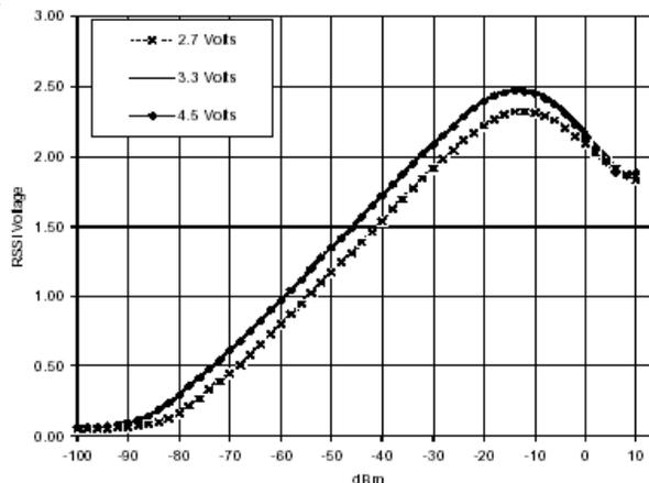
Figure 2a. RSSI Output Voltage vs Input Signal Level
