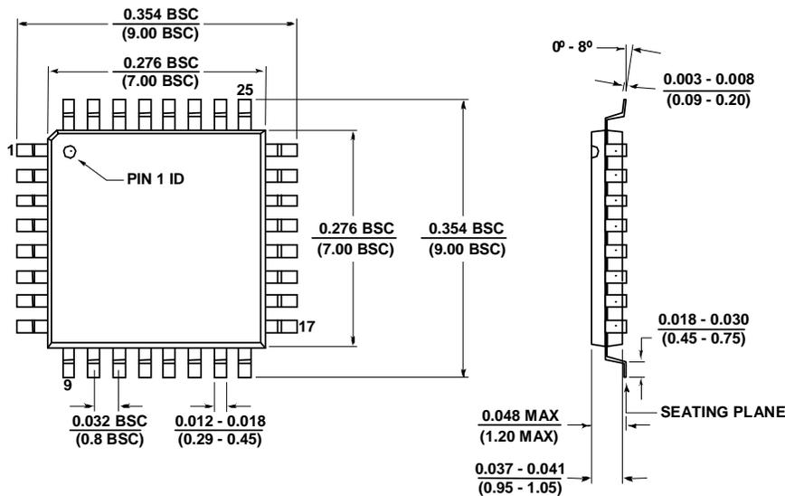
Note: This package meets “Green” Pb-Free requirements and is compliant with the European Union directives WEEE (Waste Electrical and Electronic Equipment) and RoHS (Restriction of the use of certain Hazardous Substances in electrical and electronic equipment). The package pins are finished with 100% matte tin.
