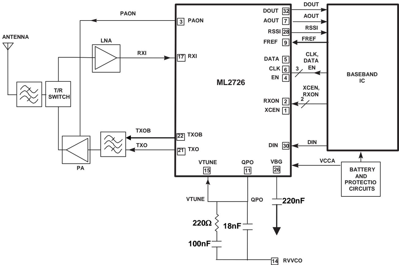
Figure 1: Typical ML2726 Application Diagram
