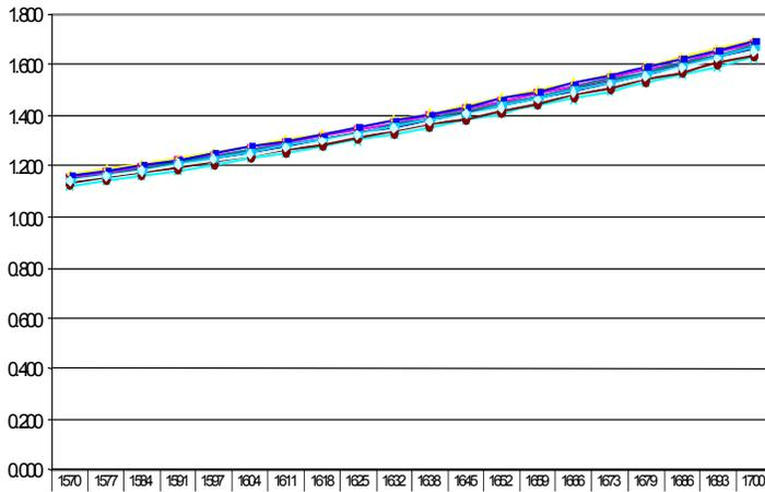
Figure 7: Typical VCO Tuning Voltage vs. Frequency
