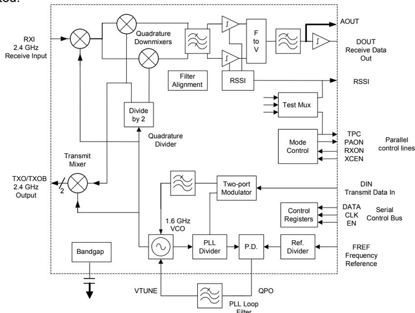
**Figure 2: ML2726 Internal Block Diagram**
