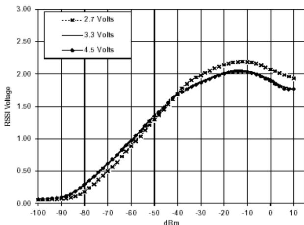
Figure 2. RSSI Output Voltage vs Input Signal Level
