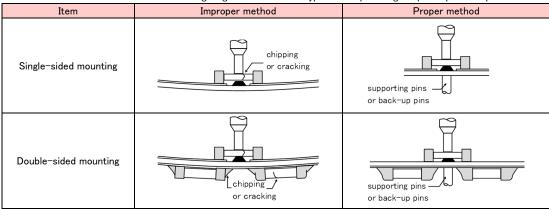
2. As the alignment pin wears out, adjustment of the nozzle height can cause chipping or cracking of the inductors because of mechanical impact on the inductors. To avoid this, the monitoring of the width between the alignment pin in the stopped position, and maintenance, inspection and replacement of the pin should be conducted periodically.
