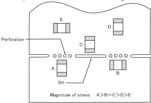
3. When breaking PC boards along their perforations, the amount of mechanical stress on the inductors can vary according to the method used. The following methods are listed in order from least stressful to most stressful: push-back, slit, V-grooving, and perforation. Thus, any ideal SMD inductor layout must also consider the PCB splitting procedure.
