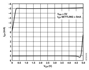
Figure 16. Charge Pump Output Characteristics
