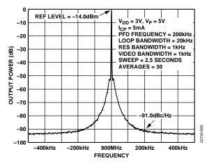
Figure 9. Reference Spurs (900 MHz, 200 kHz, and 20 kHz)
