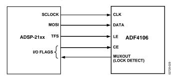
Figure 24. ADSP-21xx-to-ADF4106 Interface
