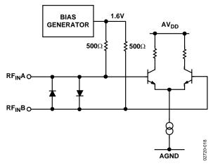
Figure 18. RF Input Stage
