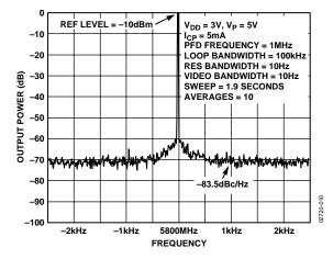
Figure 10. Phase Noise (5.8 GHz,1 MHz, and 100 kHz)
