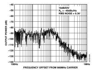
Figure 8. Integrated Phase Noise (900 MHz, 200 kHz, and 20 kHz)
