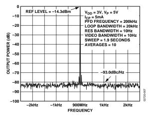
Figure 7. Phase Noise (900 MHz, 200 kHz, and 20 kHz)
