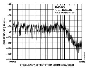
Figure 11. Integrated Phase Noise (5.8 GHz,1 MHz, and 100 kHz)
