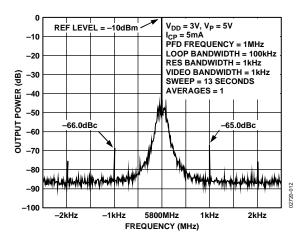
Figure 12. Reference Spurs (5.8 GHz,1 MHz, and 100 kHz)
