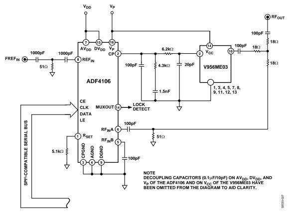
Figure 22. Local Oscillator for LMDS Base Station
