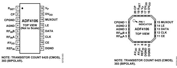
Figure 3. 16-Lead TSSOP Pin Configuration
