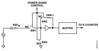
Figure 17. Reference Input Stage
