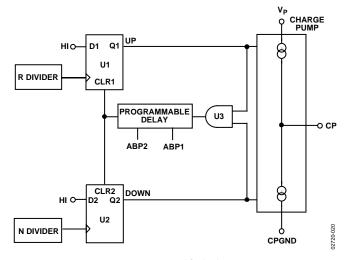
Figure 20. PFD Simplified Schematic
