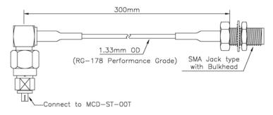
Note: For "SMA Plug" fitting, specify Pn MCD-TP-300-SMAP205
