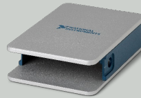
cDAQ-9171 (1-Slot CompactDAQ Chassis)
