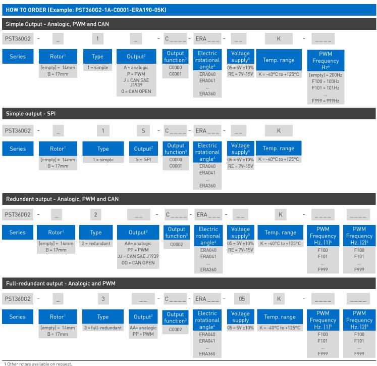
2 The analog output is ratiometric, proportional: - for supply voltage "5V" to input voltage; -for supply voltage "RE" to 5V. 3 Other output functions available, please check availability. Enter CXXXX as long as the new output function is not defined.
