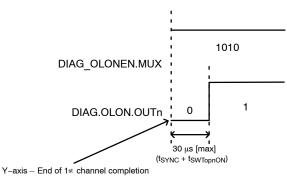
Figure 28. Subsequent Channel Loop Delay Times
