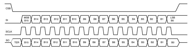
Figure 37. Serial Peripheral Interface
