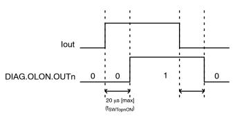
Figure 26. Direct Channel Event Delay Time
