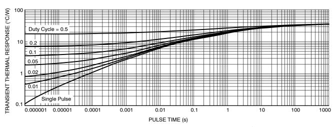
Figure 40. Transient R(t) vs. Pulse Time (JESD51-7, 600 mm²)
