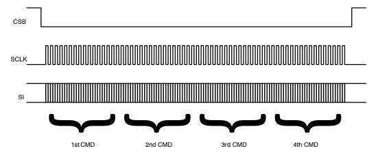
Figure 34. Serial Daisy Chain Timing Diagram
