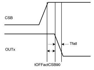
Figure 4. Serial Turn On
