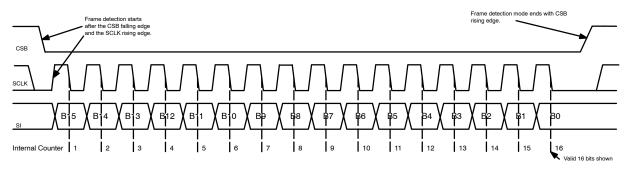
Figure 38. Frame Detection
