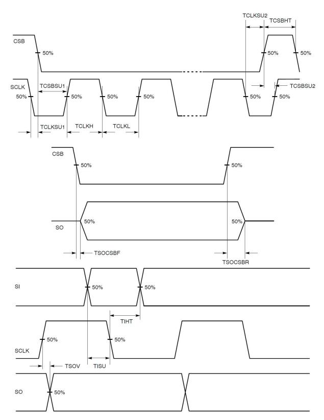
Figure 8. Serial Peripheral Interface Detailed Timing
