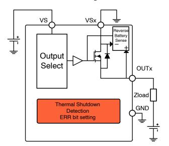
Figure 31. Reverse Polarity Control
