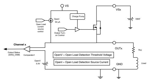
Figure 23. Open Load at OFF
