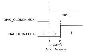
Figure 27. First Direct Channel Diagnostic Completion Timing
