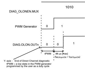
Figure 29. First MUX Channel diagnostic Completion Timing
