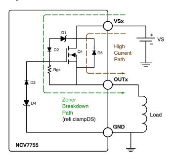
Figure 21. Output Clamp (at High Voltage)
