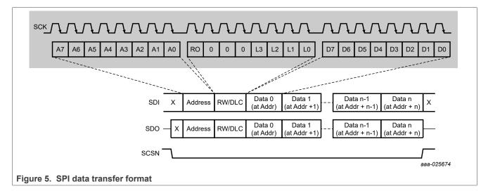
The SJA1124 monitors the number of data bits transmitted. If the number of bits is not between 24 and 144, is not a factor of 8, or the number of bytes does not match the DLC in the SPI conrol byte, the write access is ignored and an SPI error interrupt (SPIEI) is triggered (see <u>Table 22</u>).
