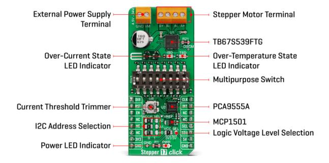
Thanks to the many steps that TB67S539FTG supports, motor noise can be significantly reduced with smoother operation and more precise control. It is suited to a wide range of applications such as office automation, commercial, and industrial equipment using stepping motors supporting an operational temperature range covering -20°C to +85°C. The current value is set by the reference
