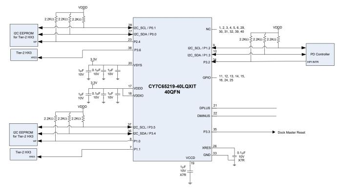
Figure 5. Dock/Monitor Application Diagram (40-QFN Device)
