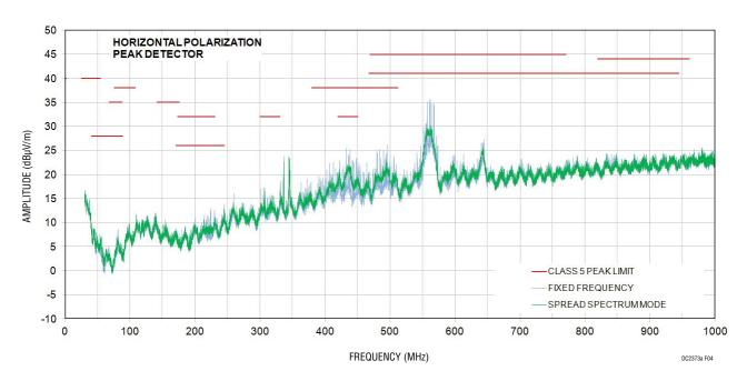
Figure 4. LT8641 Demo Circuit EMI Performance in CISPR25 Radiated Emission Test, Antenna Polarization: Horizontal ( $V_{IN} = 14V$ ,  $V_{OUT} = 5V$ ,  $I_{OUT} = 3.5A$ , 2MHz Switching Frequency)
