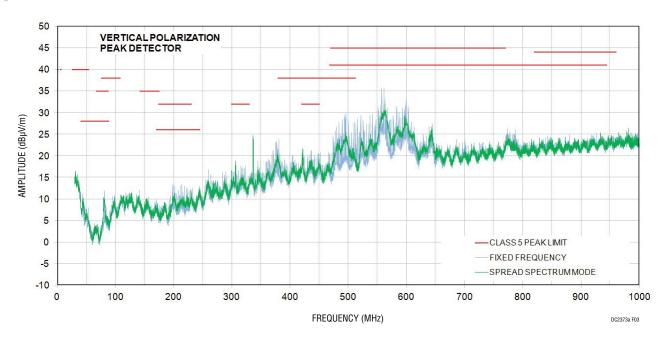
Figure 3. LT8641 Demo Circuit EMI Performance in CISPR25 Radiated Emission Test, Antenna Polarization: Vertical ( $V_{IN} = 14V$ ,  $V_{OUT} = 5V$ ,  $I_{OUT} = 3.5A$ , 2MHz Switching Frequency)
