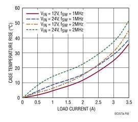
Figure 2. DC2373A Temperature Rising vs Load Current
