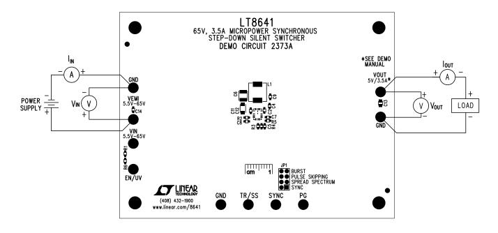
Figure 5. Proper Measurement Equipment Setup
