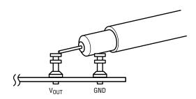
Figure 6. Measuring Output Ripple
