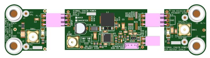
Figure 2. Proper Measurement Equipment Setup (Use SMA connectors for Measuring Input or Output Ripple)
