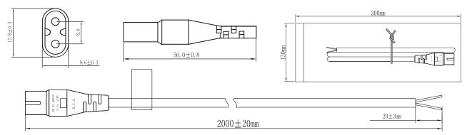
CABLE MARKING: H03VVH2-F 2X0.75mm² ⟨VDE⟩N19626 CCC A030116 No. 2003010105097406 227 IEC 52(RVV) 300/300V 2X0.75mm²
