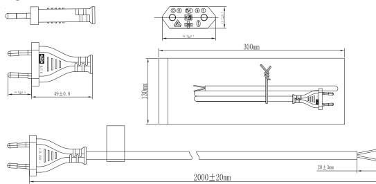
CABLE MARKING: H03VVH2-F 2X0.75mm<sup>2</sup> ⊲VDE⊳N19626 CCC A030116 No. 2003010105097406 227 IEC 52 (RVV) 300/300V 2X0.75mm<sup>2</sup>
