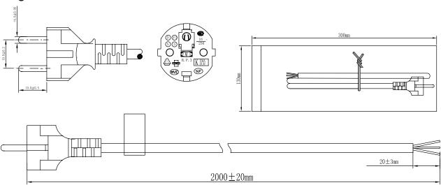
CABLE MARKING: H05VV-F 3G1.0mm² ◀ VDE ▷ N19626 CCC A030116 No. 2003010105097406 227 IEC 53 (RVV) 300/500V 3X1.0mm²
