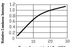
Forward current (mA) Ta=25°C Luminous Intensity vs. Forward current
