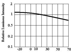
$\label{eq:ambient} \begin{tabular}{ll} Ambient Temperature $Ta$= $^{\circ}$C \\ Luminous Intensity vs. Ambient Temperature \\ \end{tabular}$
