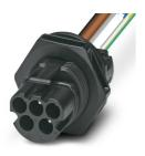
Panel feed-through, Range of articles: PRC 35, Device connector, rear mounting, housing material: PPE, color: black, number of positions: 5, max. conductor cross section: 6 mm<sup>2</sup>, rated voltage: 690 V AC, rated current: 35 A, Connection method: Crimp connection, Type of contact: Pin, cable length: 150. This item is also available with other cable lengths. For your specific requirements, please contact your local PHOENIX CONTACT subsidiary.
