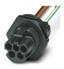
Panel feed-through, Range of articles: PRC 35, Device connector, rear mounting, housing material: PPE, color: black, number of positions: 5, max. conductor cross section: 6 mm<sup>2</sup>, rated voltage: 690 V AC, rated current: 35 A, Connection method: Crimp connection, Type of contact: Pin, cable length: 150. This item is also available with other cable lengths. For your specific requirements, please contact your local PHOENIX CONTACT subsidiary.
