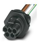
Panel feed-through, Range of articles: PRC 35, Device connector, rear mounting, housing material: PPE, color: black, number of positions: 5, max. conductor cross section: 6 mm², rated voltage: 690 V AC, rated current: 35 A, Connection method: Crimp connection, Type of contact: Pin, cable length: 150. This item is also available with other cable lengths. For your specific requirements, please contact your local PHOENIX CONTACT subsidiary.
