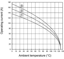
① Conductor cross-section 16 mm<sup>2</sup>
