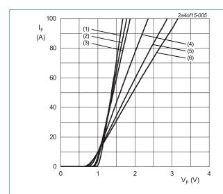
$V_{o}$  = 1.252 V;  $R_{s}$  = 0.0206  $\Omega$
