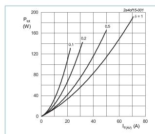
$\begin{aligned} I_{F(AV)} &= I_{F(RMS)} \times \sqrt{\delta} \\ V_o &= 1.252 \text{ V}; \text{ R}_s = 0.0206 \ \Omega \end{aligned}$  Fig. 1. Forward power dissipation as a function of average forward current; square waveform; maximum values
