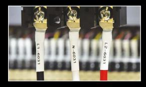
This special non-adhesive tape is made of a special material that is wound in the tape cassette as a flat tube. Once printed with the relevant identification details, the tube is opened up and passed over a cable or terminating connector. Once heated using a heat gun, the tube shrinks to about half its original width, and in doing so grips the cable.
