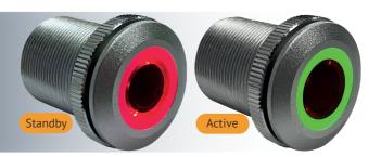
The CTL-SW is a touchless infrared proximity switch, which sits inside a Ø22mm natural anodised aluminium shell. Easily and reliably activated without contact, this proximity switch has a pre-set\* detection range of 4cm. The CTL-SW has onboard LED's showing red when the switch is in standby and green when activated. The momentary action is pre-set\* to 10 seconds.
