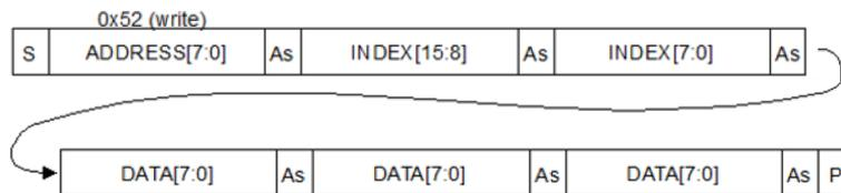
**Figure 15. VL53L8CX data format (sequential read)**
