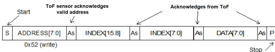
As data are received by the slave, they are written bit by bit to a serial/parallel register. After each data byte has been received by the slave, an acknowledge is generated, the data are then stored in the internal register addressed by the current index.
