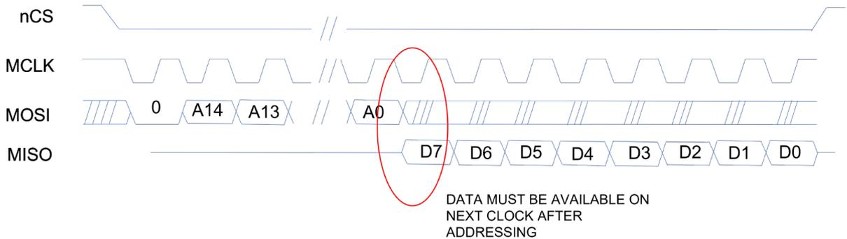
If the host continues to toggle the MCLK after the last data bit has been read, the slave goes into auto-increment read mode. In this mode, the address is automatically incremented by the slave, and the read data are transmitted sequentially to the master on the MISO line. More details of the SPI auto-increment read mode are shown in [Figure 20. SPI auto-increment read sequence](#).
