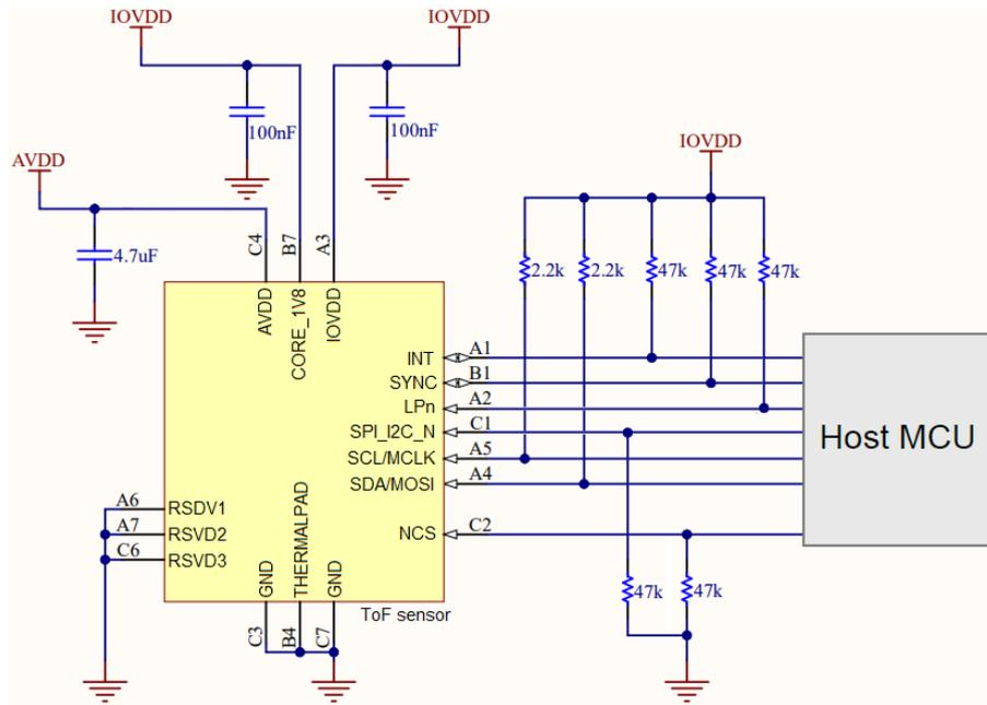
**Note:** Capacitors on the external supplies (AVDD, CORE\_1V8, and IOVDD) should be placed as close as possible to the module pins.
