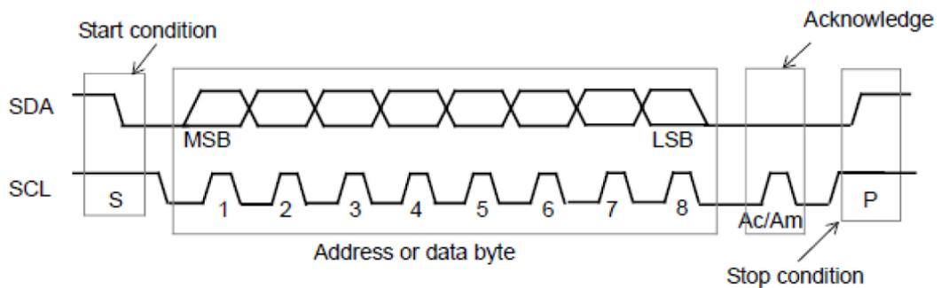
Information is packed in 8-bit packets (bytes) always followed by an acknowledge bit, Ac for VL53L8CX acknowledge and Am for master acknowledge (host bus master). The internal data is produced by sampling SDA at a rising edge of SCL. The external data must be stable during the high period of SCL. The exceptions to this are start (S) or stop (P) conditions when SDA falls or rises respectively, while SCL is high.
