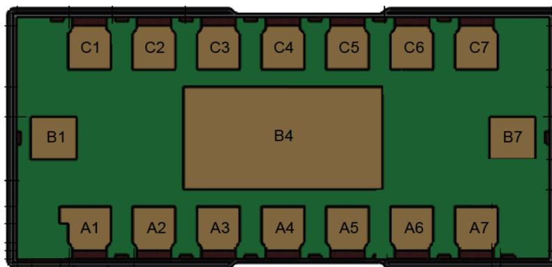
The VL53L8CX pin description for the I<sup>2</sup>C and SPI configuration is given in [Table 3. VL53L8CX pin description for I<sup>2</sup>C and SPI configuration](#). For the pins that support both I<sup>2</sup>C and SPI protocol, the I<sup>2</sup>C description is listed first and the SPI second.
