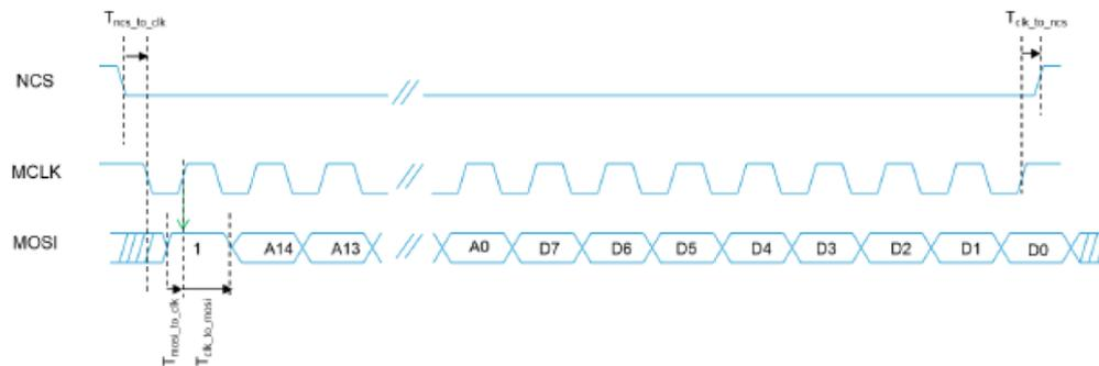
If the host continues to transmit data beyond the first 8 data bits, then the slave goes into auto-increment write mode. The auto-increment write timing sequence is shown in [Figure 18. SPI auto-increment write sequence](#). The MOSI initial value is 1. The address is incremented automatically and internally by the slave. Subsequent data bits correspond to incrementing addresses.
