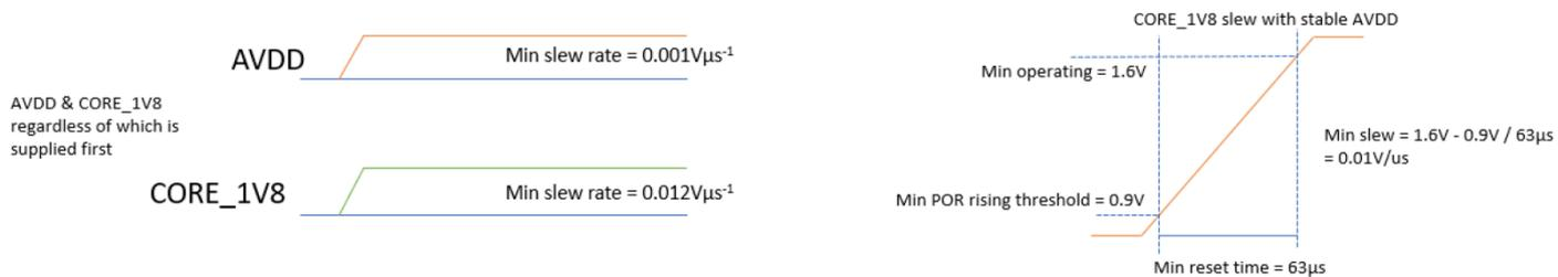
**Note:** The minimum reset time is the minimum time required for the device RAM to load and boot up after CORE\_1V8 reaches the power-on reset rising threshold. The supply must have reached the minimum operating level (1.6 V) within this time.
