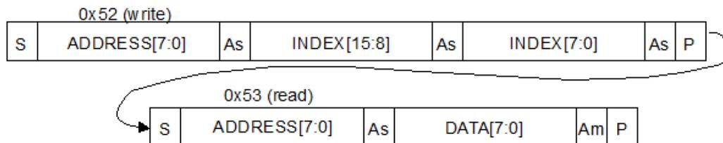
At the end of each byte, in both read and write message sequences, an acknowledge is issued by the receiving device (that is, the VL53L8CX for a write and the host for a read).
