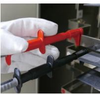
For clamping around the target busbar
