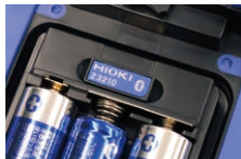
Attach to enable Bluetooth® wireless technology
