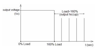
Additionally, if the 12 Volts' lout is >100%; but <160% for a prolonged period of time (depending on the load), the Over Temperature Protection (OTP) will be activated due to high temperature on critical components. The power supply will then go into latch mode.
