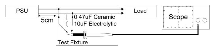
Fig. 3 Ripple & Noise measurement circuit
