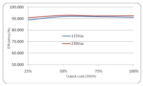
Fig.1 Efficiency versus output load
