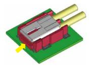
(2) Continue to rotate it upwards and release the friction lock portion.
