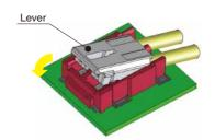
(3) Keep pressing down until a "click" feeling is sensed. The connector is now fully and properly mated.
