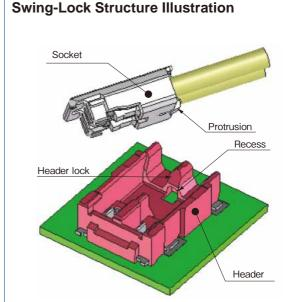
The protrusion on the bottom side of the socket fits into a corresponding recess on the header. This aligns the socket into the correct mating position.
