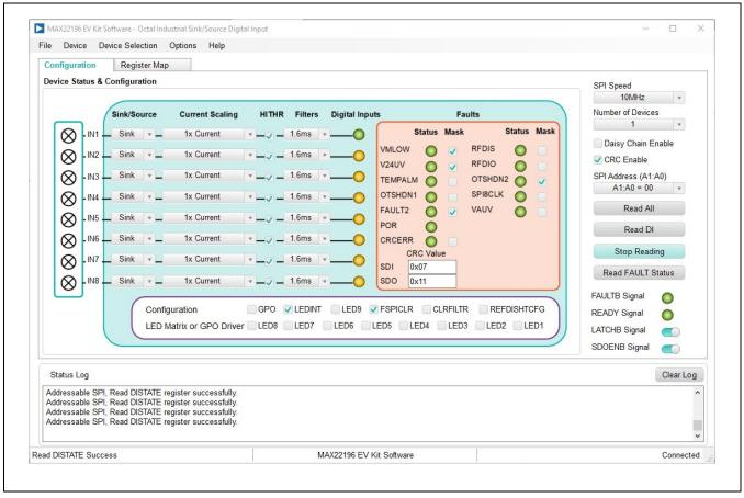
Figure 2. MAX22196 EV Kit Software—Type 1/3 Sink Mode Configuration
