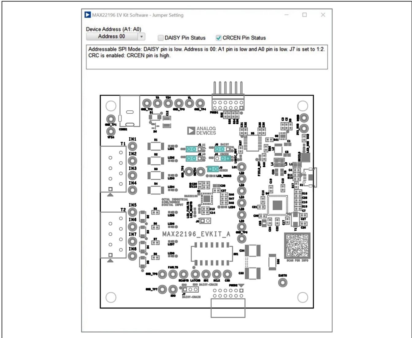
Figure 5. MAX22196 EV Kit Software—Jumper Setting Diagram
