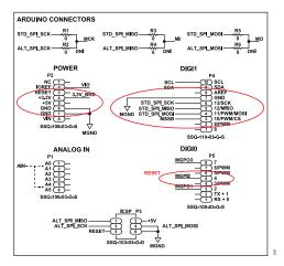
Figure 19. Arduino Connector During User-Defined SPI Setup
