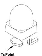
$T_S$  can be easily measured by mounting a thermocouple on the soldering joint as shown in Figure 12, while  $R\theta_{J\text{-}S}$  is provided in this data sheet. Verify the  $T_S$  of the LED in the final product to ensure that the LEDs are operating within all maximum ratings stated in this data sheet.
