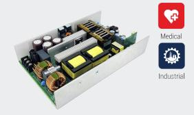
Advanced Energy's SL Power NGB800 series of open-frame AC-DC power supplies features ITE and medical safety approvals. The series offers a choice of four single output models, with voltages of 12 V, 15 V, 24 V, or 48 V. Each model also provides an isolated 12 V fan output, and 5 V standby output. NGB800 series power supplies provide 800 Watts of output power, and have a typical full load power conversion
