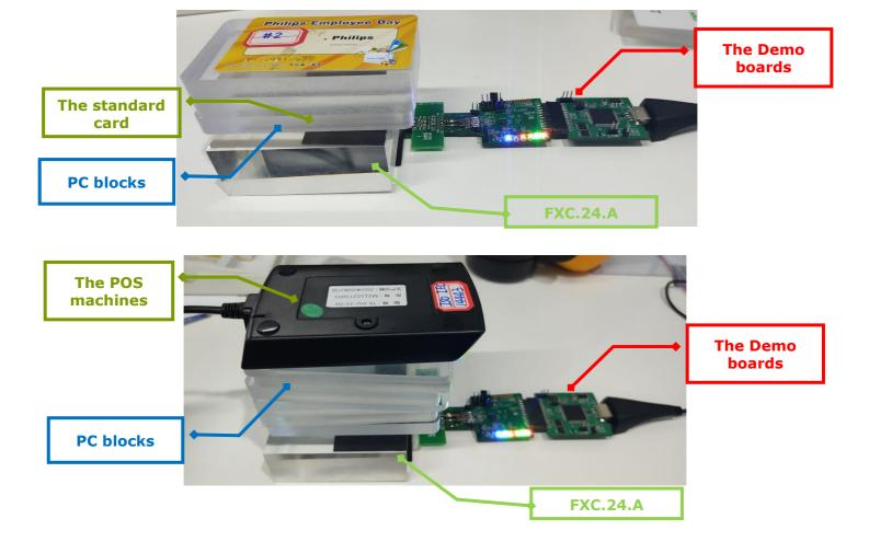
When the number of the PC material blocks are carefully adjusted until the reader can no longer read the sample, that's mean in this point the FXC.24.A cannot establish communication with the standard card or the POS machine, the thickness of the PC material block is the maximum interrogation distance of them.
