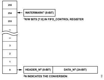
Figure 102. FIFO Structure
