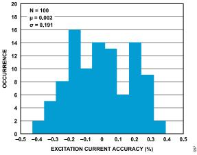
Figure 57. Excitation Current Initial Accuracy Histogram (100 µA)
