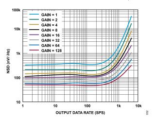
Figure 32. NSD vs. Output Data Rate for Various Gains (Sinc<sup>3</sup> Filter, External 2.5 V Reference)
