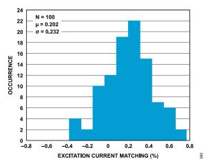
Figure 60. Excitation Current Initial Matching Histogram (100 µA)
