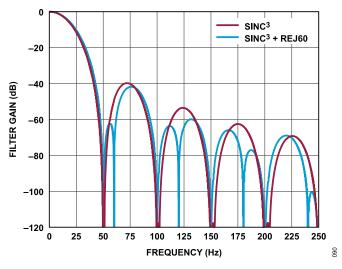
Figure 90. Sinc<sup>3</sup> and Sinc<sup>3</sup> + REJ60 Filter Response (50 SPS ODR)
