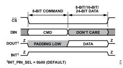
Figure 74. Reading from a Register (8-Bit Command with Register Address Followed by Data)
