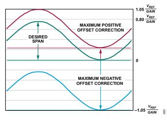
Figure 83. Example of Unipolar Span and Offset Calibration Limits
