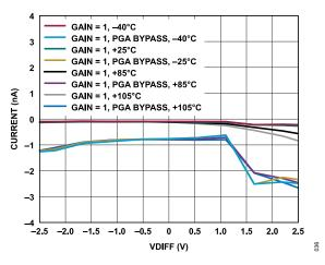
Figure 36. Absolute AINM Current vs. VDIFF for Various Temperatures (Gain = 1, VCM = AV<sub>DD</sub>/2)
