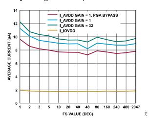
Figure 46. Duty Cycling Current Consumption ( $AV_{DD}$  and  $IOV_{DD}$ ), DUTY\_CYC\_RATIO = 1/4 (I\_AVDD is  $AV_{DD}$  Current, I\_IOVDD is  $IOV_{DD}$  Current)
