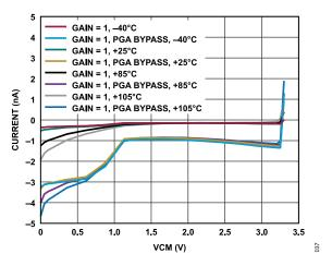
Figure 37. Absolute AINM Current vs. VCM for Various Temperatures (Gain = 1, VDIFF = 0 V)
