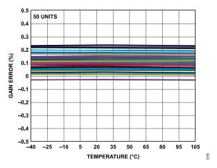
Figure 19. Gain Error vs. Temperature (Gain = 8, Before Calibration)
