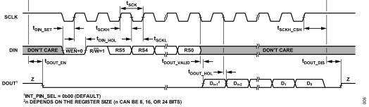
Figure 6. 3-Wire Mode Read Cycle Timing Diagram, 3-Wire Mode (CSB\_EN Bit Set to 0), CS Pin Used to Tristate the DOUT Pin
