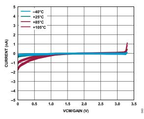
Figure 43. Absolute AINM Current vs. VCM/Gain for Various Temperatures (Gain = 2 to 128, VDIFF = 0 V)
