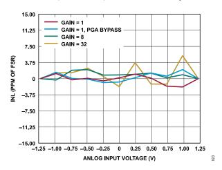
Figure 23. INL Error vs. Differential Input Amplitude for Various Gains (Sinc<sup>3</sup> Filter, ODR = 50 SPS, AV<sub>DD</sub> = 1.8 V, Internal 1.25 V Reference)
