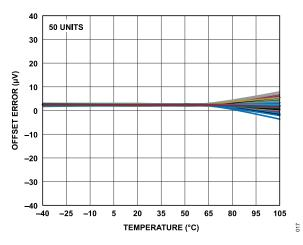
Figure 17. Offset Error vs. Temperature (Gain = 32, Before Calibration)
