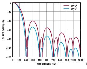
Figure 85. Sinc<sup>3</sup> and Sinc<sup>4</sup> Filter Response (FS = 0d10)
