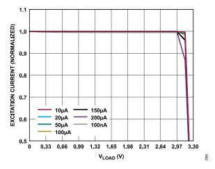
Figure 59. Output Compliance for Various IEXC Sources (AV<sub>DD</sub> = 3.3 V, V<sub>LOAD</sub> is Load Voltage)
