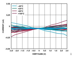
Figure 41. Differential AIN Current vs. VDIFF/Gain for Various Temperatures (Gain = 2 to 128, VCM = AV<sub>DD</sub>/2)
