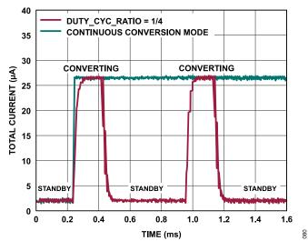
Figure 80. Example of Duty Cycling Mode vs. Continuous Conversion Mode Current Consumption
