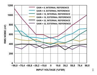
Figure 31. RMS Noise vs. Analog Input Voltage (Sinc<sup>3</sup> Filter, ODR = 50 SPS, Gain = 8, Gain = 16 and Gain = 32, 2.5 V Reference)
