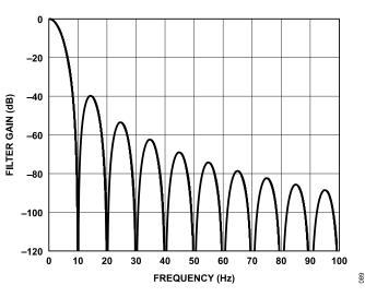
Figure 89. Simultaneous 50 Hz and 60 Hz Rejection for Sinc<sup>3</sup> with ODR = 10 SPS
