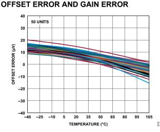
Figure 15. Offset Error vs. Temperature (Gain = 1, Before Calibration)
