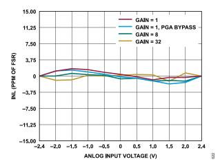
Figure 22. INL Error vs. Differential Input Amplitude for Various Gains (Sinc<sup>3</sup> Filter, ODR = 50 SPS, External 2.5 V Reference)
