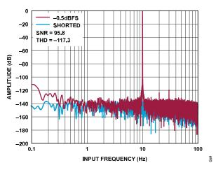
Figure 68. FFT, -0.5 dBFS vs. Shorted Inputs, 10 Hz Input Tone, Sinc<sup>3</sup> Filter, ODR = 240 SPS, Gain = 1, External Reference
