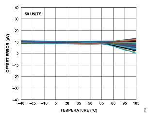
Figure 16. Offset Error vs. Temperature (Gain = 8, Before Calibration)
