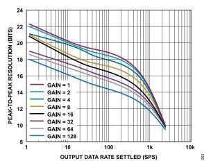
Figure 63. Peak-to-Peak Resolution vs. Output Data Rate (Settled) for Various Gains (Sinc<sup>3</sup> Filter)
