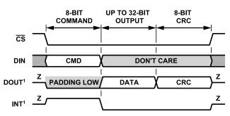
Figure 99. SPI Write Transaction with CRC
