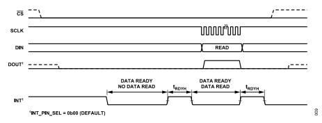
Figure 9. Data Ready High Time when Data Ready is Initially Low and the Next Conversion is Available
