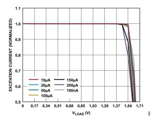
Figure 62. Output Compliance for Various IEXC Sources (AV<sub>DD</sub> = 1.71 V)
