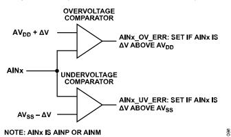
Figure 98. Analog Input Overvoltage/Undervoltage Monitors
