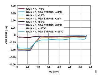
Figure 38. Differential AIN Current vs. VCM for Various Temperatures (Gain = 1, VCM = AV<sub>DD</sub>/2)
