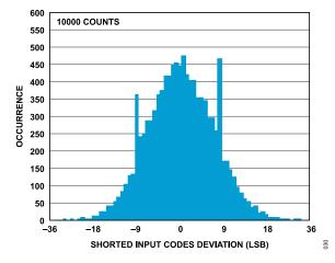
Figure 30. Noise Histogram Plot (Sinc<sup>4</sup> Filter, ODR = 240 SPS, Gain = 1, Internal 1.25 V Reference)
