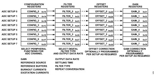
Figure 76. ADC Setup Register Grouping
