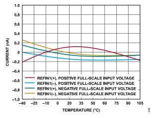
Figure 49. Reference Input Current vs. Temperature (Reference Buffer On, External 2.5 V Reference)
