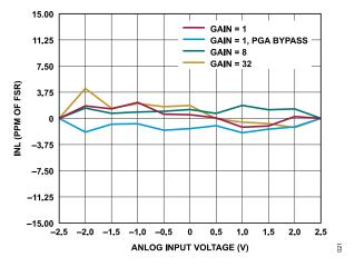
Figure 21. INL Error vs. Differential Input Amplitude for Various Gains (Sinc<sup>3</sup> Filter, ODR = 50 SPS, Internal 2.5 V Reference)
