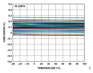
Figure 20. Gain Error vs. Temperature (Gain = 32, Before Calibration)
