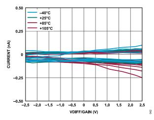
Figure 42. Absolute AINM Current vs. VDIFF/Gain for Various Temperatures (Gain = 2 to 128, VCM = AV<sub>DD</sub>/2)
