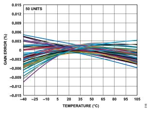
Figure 18. Gain Error vs. Temperature (Gain = 1, Factory Calibrated)
