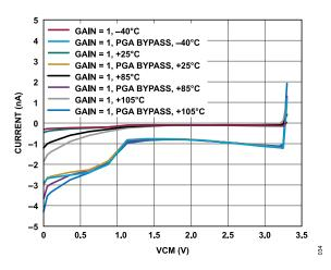
Figure 34. Absolute AINP Current vs. AIN Common-Mode Voltage (VCM) for Various Temperatures (Gain = 1, VDIFF = 0 V)
