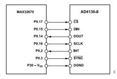
Figure 107. Example of MAX32670 µC SPI Connection to AD4130-8
