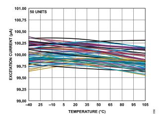
Figure 58. Excitation Current vs. Temperature (100 µA)
