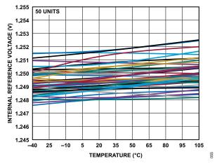
Figure 55. 1.25 V Internal Reference Voltage vs. Temperature
