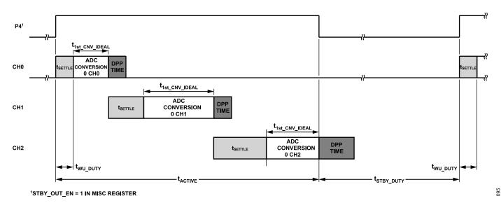
Figure 95. Example of Autonomous Duty Cycling Mode
