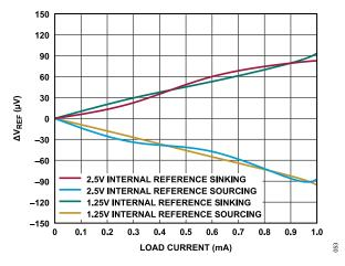
Figure 53. 1.25 V (AV<sub>DD</sub> = 1.8 V) and 2.5 V (AV<sub>DD</sub> = 3.3 V) Internal Reference Voltage vs. Load Current
