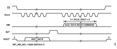
Figure 82. Exit Continuous Read Mode Diagram (CRC Disabled)
