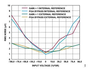
Figure 28. RMS Noise vs. Analog Input Voltage (Sinc<sup>3</sup> Filter, ODR = 50 SPS, Gain = 1 and Gain = 1 with PGA Bypass, 2.5 V Reference)
