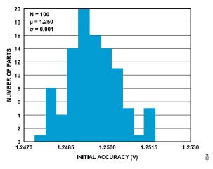
Figure 54. 1.25 V Internal Reference Voltage Histogram
