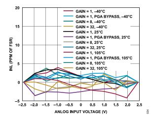
Figure 24. INL Error vs. Differential Input Amplitude for Various Gains and Temperatures (Sinc<sup>3</sup> Filter, ODR = 50 SPS, Internal 2.5 V Reference)
