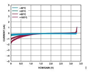
Figure 40. Absolute AINP Current vs. Normalized AIN Common-Mode Voltage (VCM/Gain) for Various Temperatures (Gain = 2 to 128, VDIFF = 0 V)
