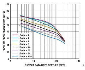
Figure 64. Peak-to-Peak Resolution vs. Output Data Rate (Settled) for Various Gains (Sinc<sup>3</sup> + Sinc<sup>1</sup> Filter)
