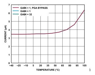
Figure 47. IOV<sub>DD</sub> Current vs. Temperature
