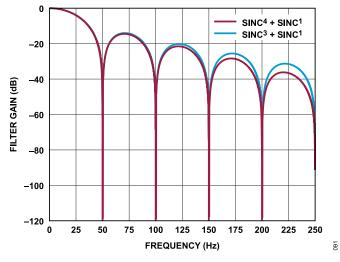
Figure 91. Sinc<sup>3</sup> + Sinc<sup>1</sup> and Sinc<sup>4</sup> + Sinc<sup>1</sup> Filter Response (FS = 6)
