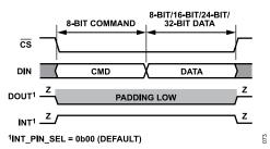
Figure 73. Writing to a Register (8-Bit Command with Register Address Followed by Data)
