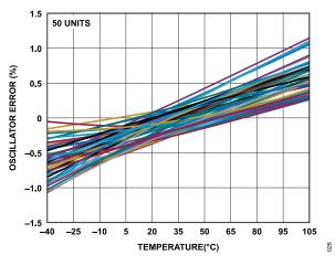
Figure 26. Internal Oscillator Error vs. Temperature
