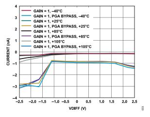
Figure 33. Absolute AINP Current vs. Differential AIN Voltage (VDIFF) for Various Temperatures (Gain = 1, VCM = AV<sub>DD</sub>/2)
