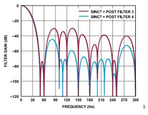
Figure 87. Post Filter 3 and Post Filter 4 Response
