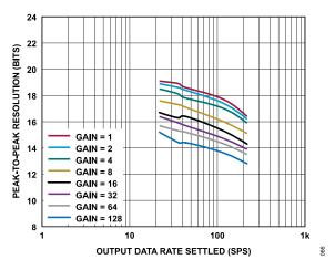
Figure 66. Peak-to-Peak Resolution vs. Output Data Rate (Settled) for Various Gains (Sinc<sup>4</sup> + Sinc<sup>1</sup> Filter)
