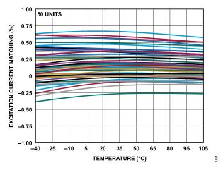
Figure 61. Excitation Current Matching vs. Temperature (100 µA)
