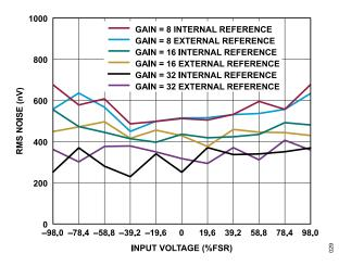
Figure 29. RMS Noise vs. Analog Input Voltage (Sinc<sup>3</sup> Filter, ODR = 50 SPS, Gain = 8, Gain = 16 and Gain = 32, 1.25 V Reference)
