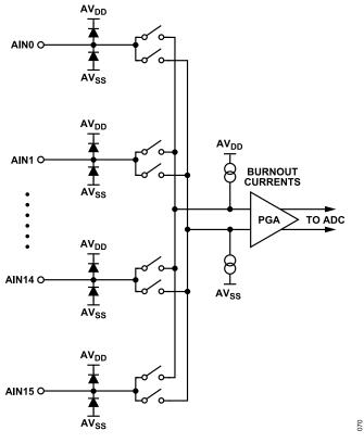
Figure 70. Analog Input Multiplexer Circuit
