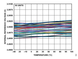
Figure 52. 2.5 V Internal Reference Voltage vs. Temperature
