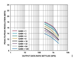
Figure 65. Peak-to-Peak Resolution vs. Output Data Rate (Settled) for Various Gains (Sinc<sup>4</sup> Filter)
