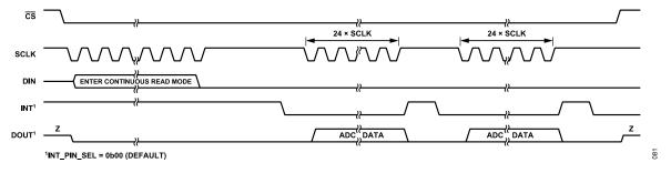
Figure 81. Enter Continuous Read Mode Diagram (DATA\_STATUS = 0)
