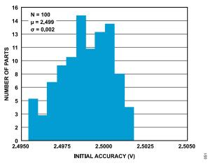
Figure 51. 2.5 V Internal Reference Voltage Histogram
