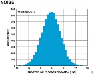
Figure 27. Noise Histogram Plot (Sinc<sup>3</sup> Filter, ODR = 50 SPS, Gain = 1)
