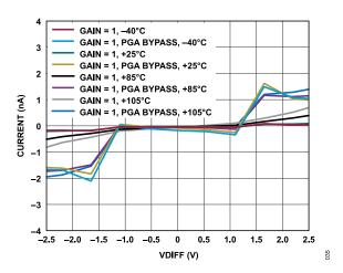
Figure 35. Differential AIN Current vs. VDIFF for Various Temperatures (Gain = 1, VCM = AV<sub>DD</sub>/2)
