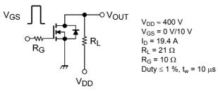
Fig. 6.2.1 Switching Time Test Circuit
